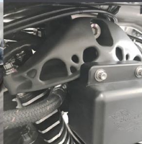
ECOSSE Motorcycle Engine Mount Bracket - 35% weight reduction
