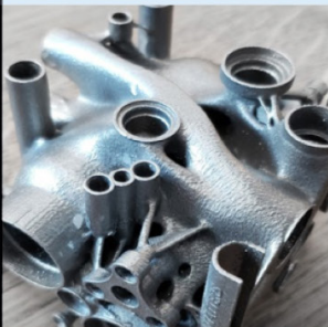
Manifold Lightweighted Design - 56% weight reduction
